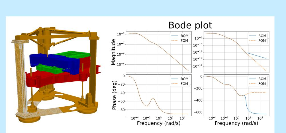
▲ Thermal Transregio 96 Model. Thermal model which describes heat induced by friction and surrounding building blocks in one of the 'z-pillars'. The full-order model coming from a FEM discretization is represented by a linear state-space system with 39,527 DOFs. A ROM with order 30 has been computed using balanced truncation.
